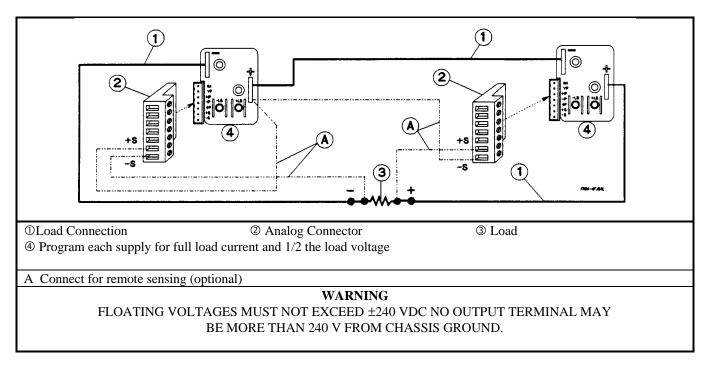
Figure 4-4f. Series 667xA Series Connection (Remote Sensing Optional)
